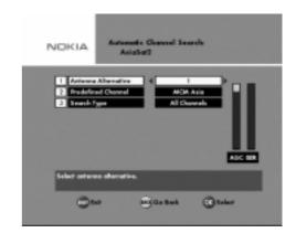
**Predefined Channel**: Each antenna alternative has one or two pre-programmed channel parameters. Choose a channel from which you want to start the channel search. Normally, each of the pre-programmed channels gives the same result.
